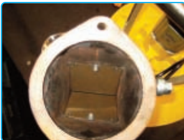
Imagine of the pump discharge mouth with windows closed
