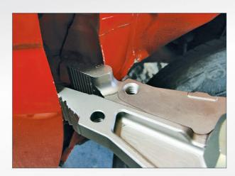
The threaded attachment points allow pulling chains to be attached
